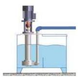
The vertical centrifugal pumps must only be installed with the axis positioned vertically and the pump immersed in the tank. Suitable devices must be used to avoid dry operation, the formation of vortexes and the possible intake of air. The vertical centrifugal pumps must only operate when the PUMP IS FLOODED; operation when dry or with air bubbles can cause damage to the internal bushing.
